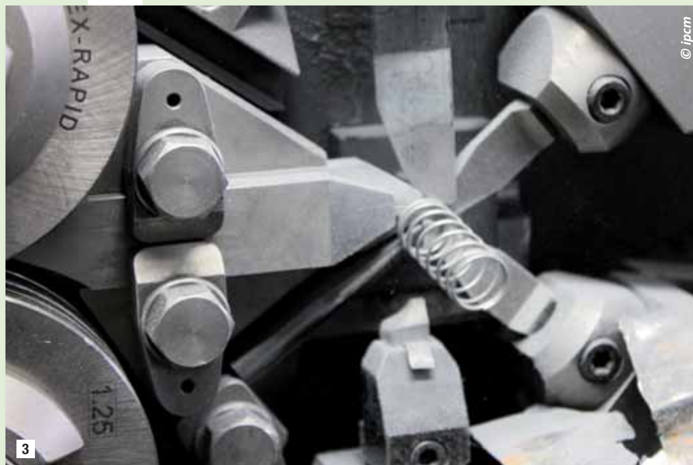
3 A detail of one of the fully automatic machines for the production of springs.
