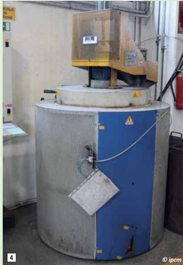
4 The oven for the heat treatment has been approved in compliance with the Nadcap specifications.
